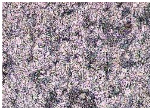
Transversal sample - Spheroidised - Little segregation
