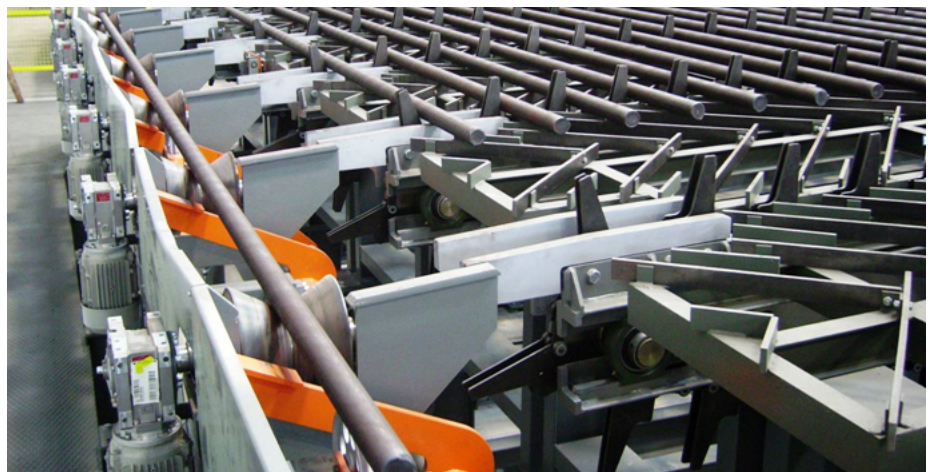
Induction heat treatment at Tre Valli Acciai division of the Lucefin Group.
