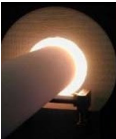
Passage through the heating coil.
