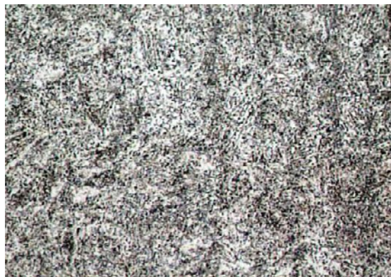
ferrite-perlite e carburi
