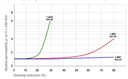
The graph shows the indicative trend of relative permeability in function of the percentage of drawing work hardening for three austenitic steels. Permeability is reduced by increasing the percentage of Nickel, Manganese, Carbon, Copper, and Nitrogen, which are elements capable of stabilizing austenite and limit the formation of martensite during the cold work hardening.
