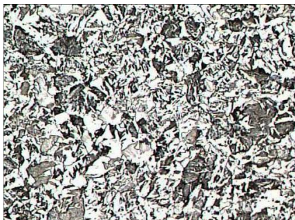
Untreated material Structure: ferrite, sorbite and bainite x200
